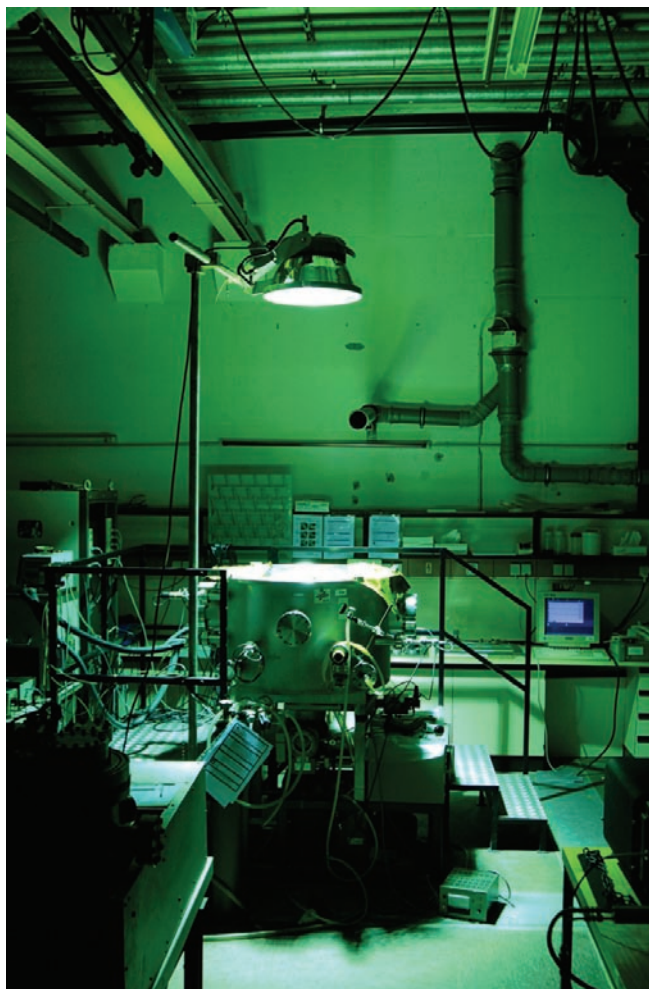
Fig. 4. Planetary and Space Simulation facility PSI 2: irradiation with solar simulator SOL2000.
