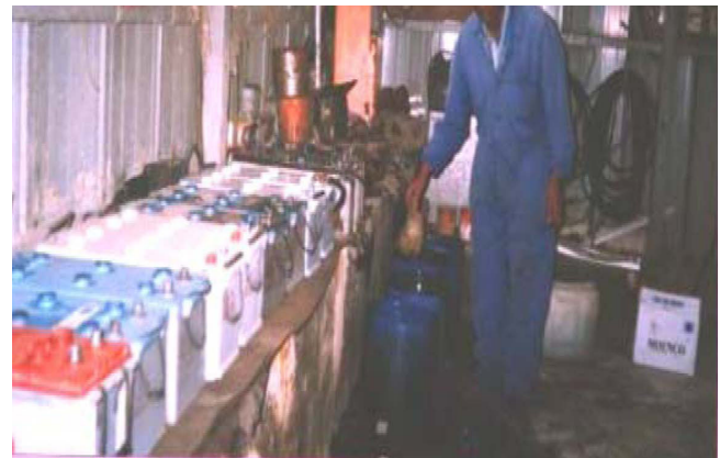
Figure 5 A partial view of storage battery repair unit in one of the enterprises. workers are engaged in routine activities without personal protective equipment, poor ventilation and full of dust.
