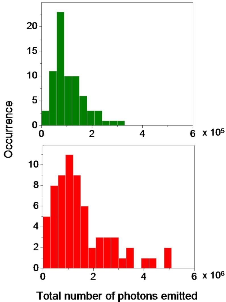
**Figure 2.** Histograms of total number of photons detected before photobleaching. Top: GFP molecules on glass (green bars) ; Bottom: GFP molecules on silver island films (red bars).
