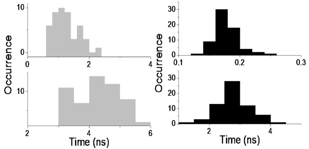
**Figure 4.** Histograms of lifetime components analyzed by bioexponential fitting to TCSPC decay curves. Left: on glass (gray bars); right: on silver island films (dark bars).
