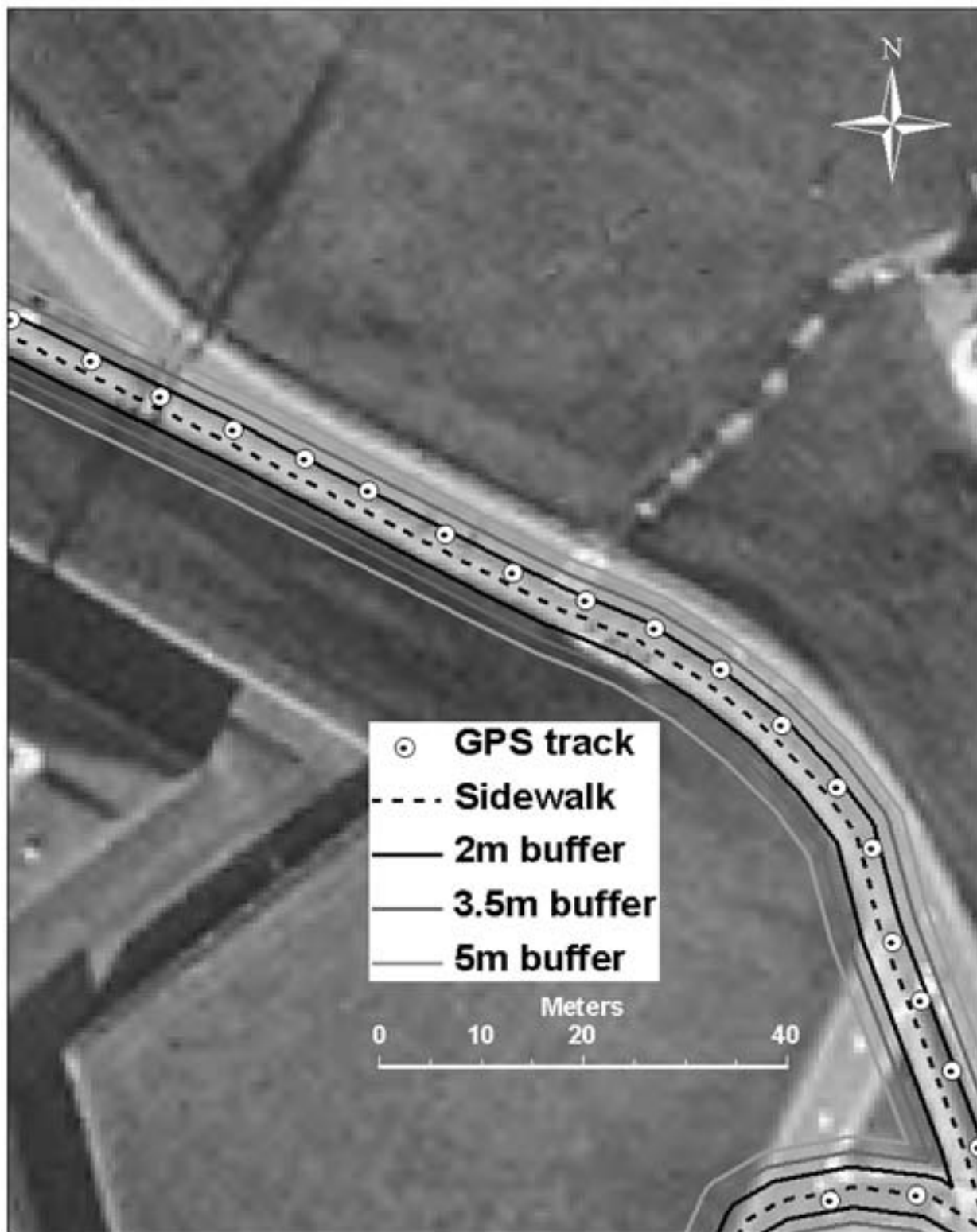
Figure 4 A sample of points logged by the GPS instrument during a 45 minute walking test in open sky or optimal reception conditions. The true path (dotted line) is the sidewalk. Most points fall within 2 m of the true path.
