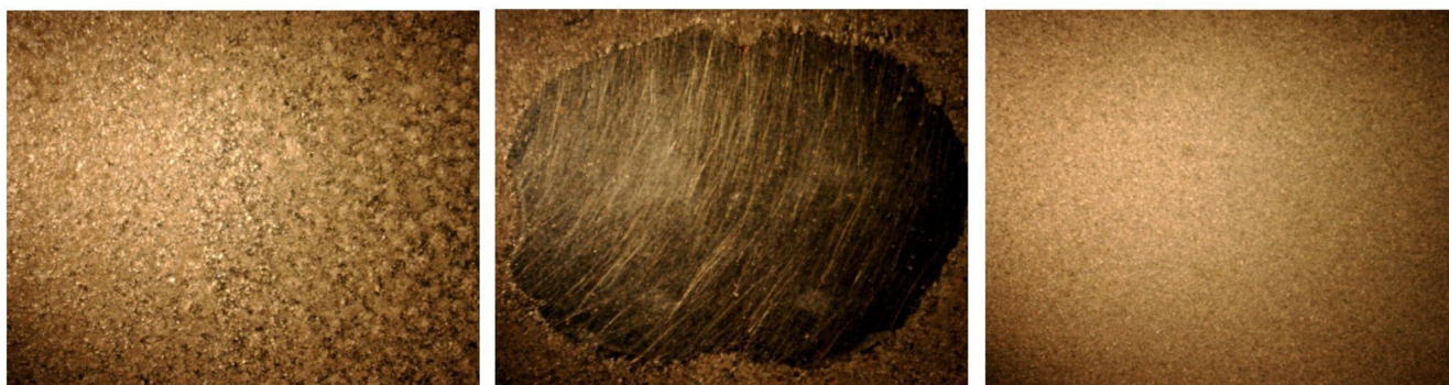
Figure 1. Surface light microscope pictures of a target plate sprayed with DHB. Left panel: Sprayed with TLC sprayer. Middle panel: Sprayed with Collision Nebulizer over a tissue section. Note the section was not covered by the matrix. Right panel: Sprayed with air brush. Note the homogeneous deposition of matrix over the target surface as compared to the TLC deposition method. Scale bar: 5 mm.
