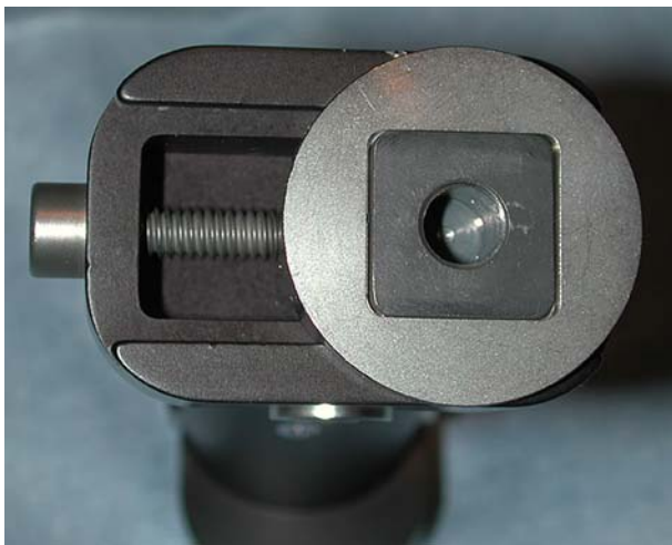
Fig. 2 There is a translation screw at either end mounted 90° to one another and each is capable of 3 cm of translation.
