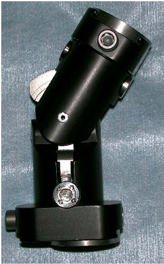
Fig. 1 The multiaxial correction system consists of a central component with a primary and secondary hinge capable of 80° and 35° to 55° of angulation, respectively, in two planes.
