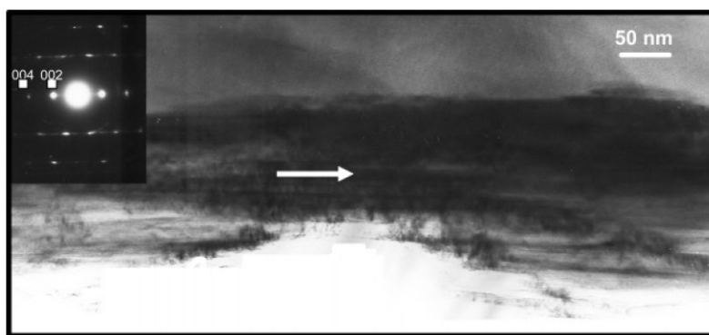
Figure 3. TEM characterization of one part of a ribbon collected after stage II (Figures 1 and 4) in a free drift nucleation experiment in the presence of 5.0 \mu\text{g mL}^{-1} Amel. The inserted SAED pattern confirmed that the ribbonlike structure was HAP. The long arrow indicates the long axis direction of the elongated microstructures.
