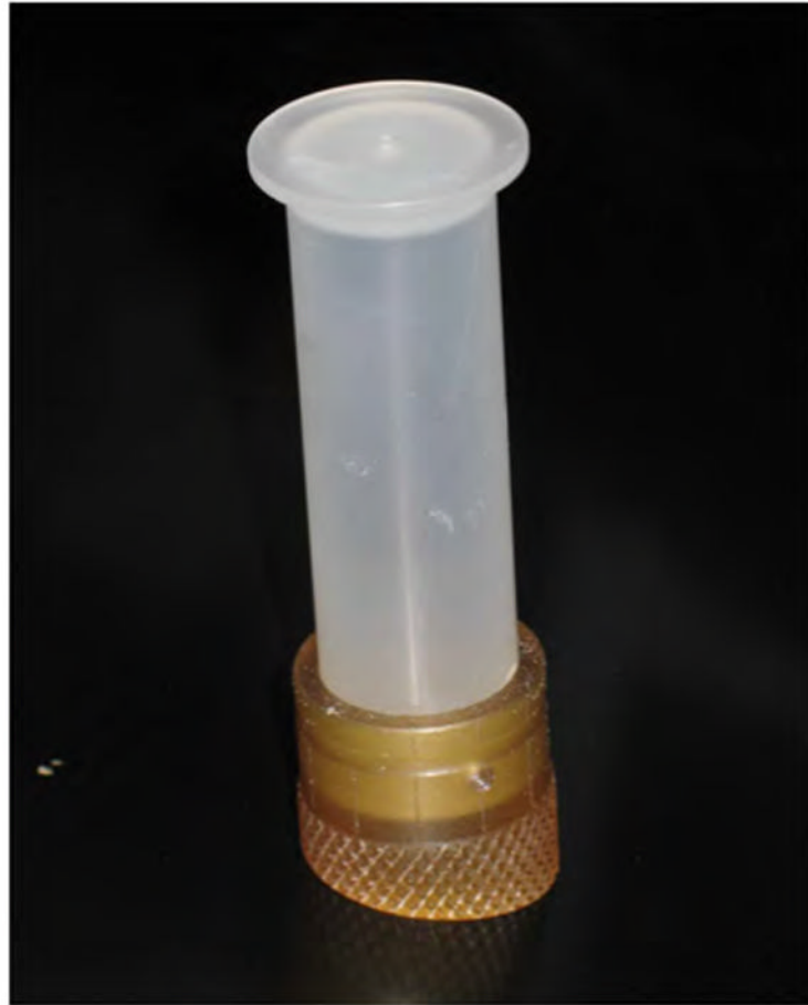
Figure 2. Recording chamber and plastic cylinder. The cylinder must fit snugly within the recording chamber so that the long axis of the cylinder is parallel to the long axis of the cylinder.
