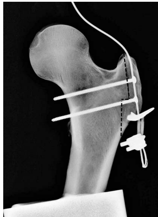
Fig. 2 Postsurgical anteroposterior radiograph of a representative step cut specimen demonstrates the cortical screws are perpendicular to the osteotomy interface and the cable is parallel to the osteotomy interface.
