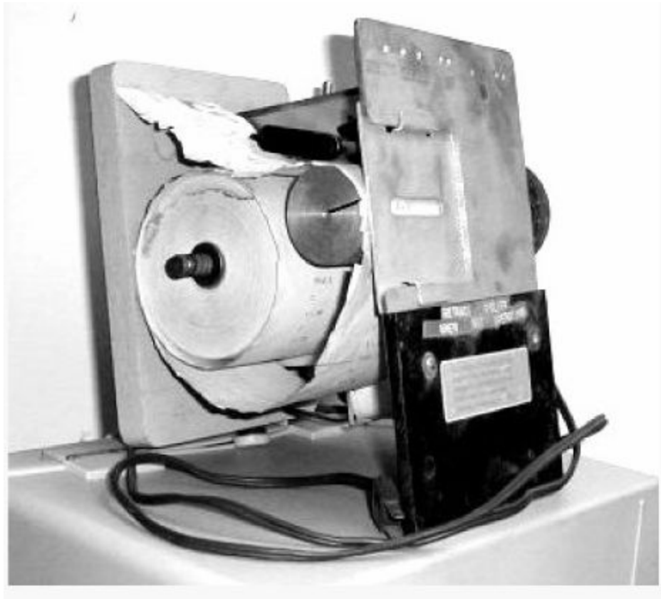
Figure 11. An early apparatus for studying verbal learning at the University of Missouri - Columbia, where John A. McGeoch was Chairmain from 1930 to 1935. An electric motor advanced the paper roll at preset intervals so that the current trial's stimuli were visible through the slot-shaped window in the metal plate shown here on the right. McGeoch (1932) advanced the idea that forgetting cannot be attributed to the passage of time per se.
