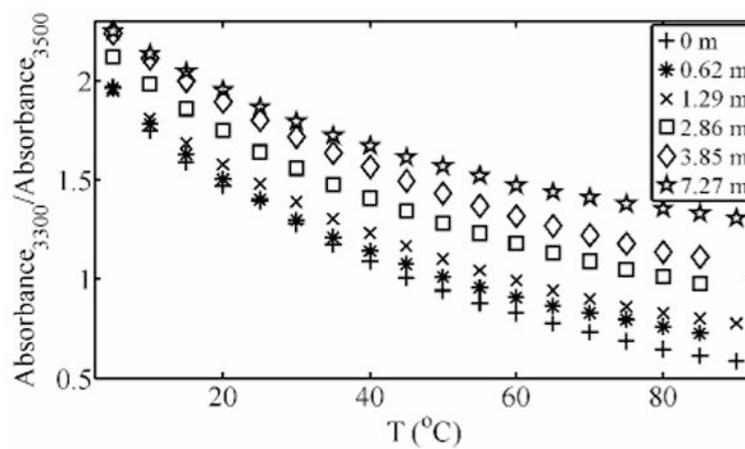
**Figure 3.** Ratio of spectral intensities at  $3300\text{ cm}^{-1}$  and  $3500\text{ cm}^{-1}$  for selected  $\text{Gdm}^+/\text{Cl}^-$  OH stretch spectra shown in Figure 1.
