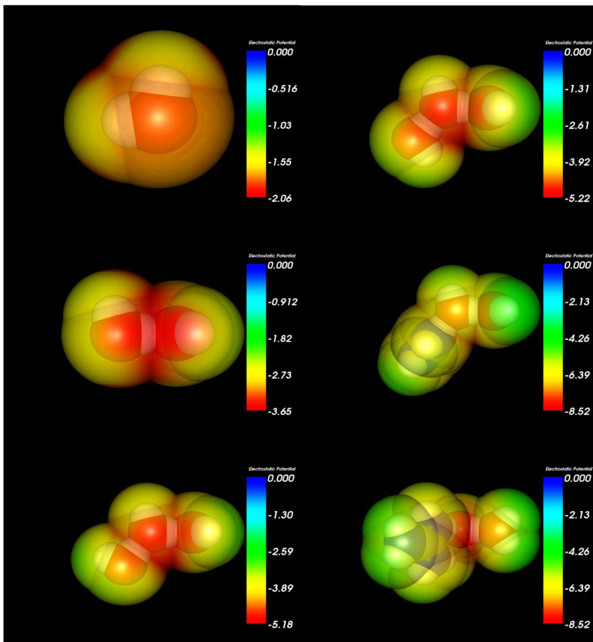
**Figure 5.** Electrostatic potential maps at the solvent accessible surface (1.4 Å solvent radius probe) generated for the water monomer and linear molecular configurations using Molekel 5.3.0.6 and colored by molecular electrostatic potential.
