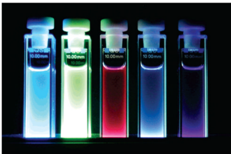
Figure 2. Photograph of ca. 10^{-4} M solutions of the free ligand (far left) and the [\text{LnR}(+)\text{BnMeH22IAM}] complexes in MeOH with Ln = Tb, Eu, Dy, Sm from left to right, respectively, upon excitation by a standard laboratory UV lamp ( \lambda_{\text{exc}} = 365 nm).
