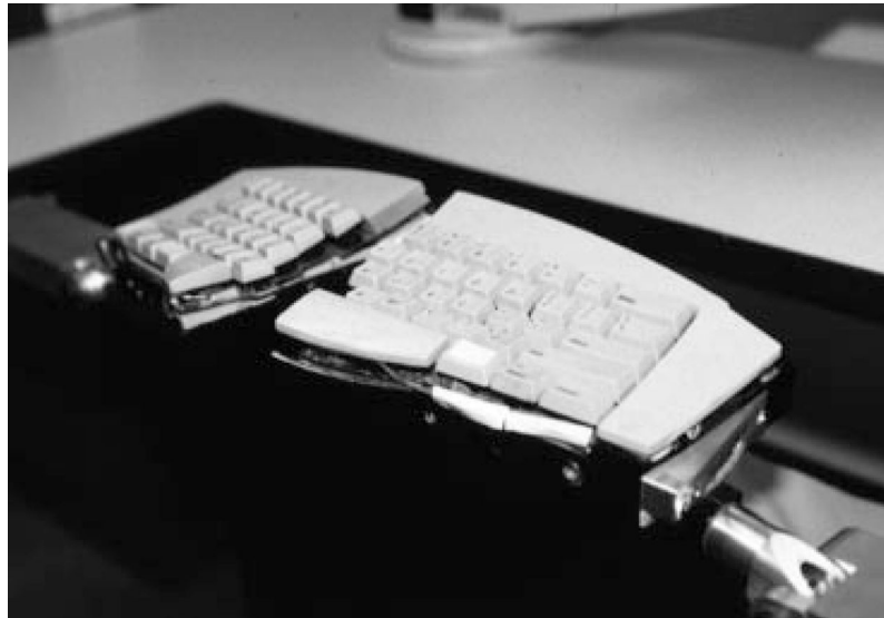
Figure 1. Custom adjustable keyboard used in study. Keyboard adjusts in height, separation of the two halves, slope (front to back), opening angle (to alter ulnar/radial deviation), and tenting or gable. In this study there was no tenting.
