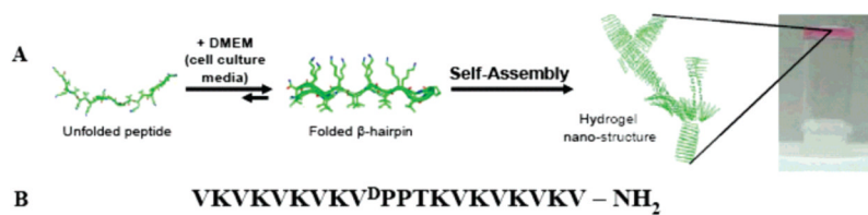
Figure 1. (A) Mechanism of folding and self-assembly for MAX1 hydrogel formation. Resulting gels are self-supporting as image at far right shows. (B) Sequence of MAX1 \beta -hairpin.
