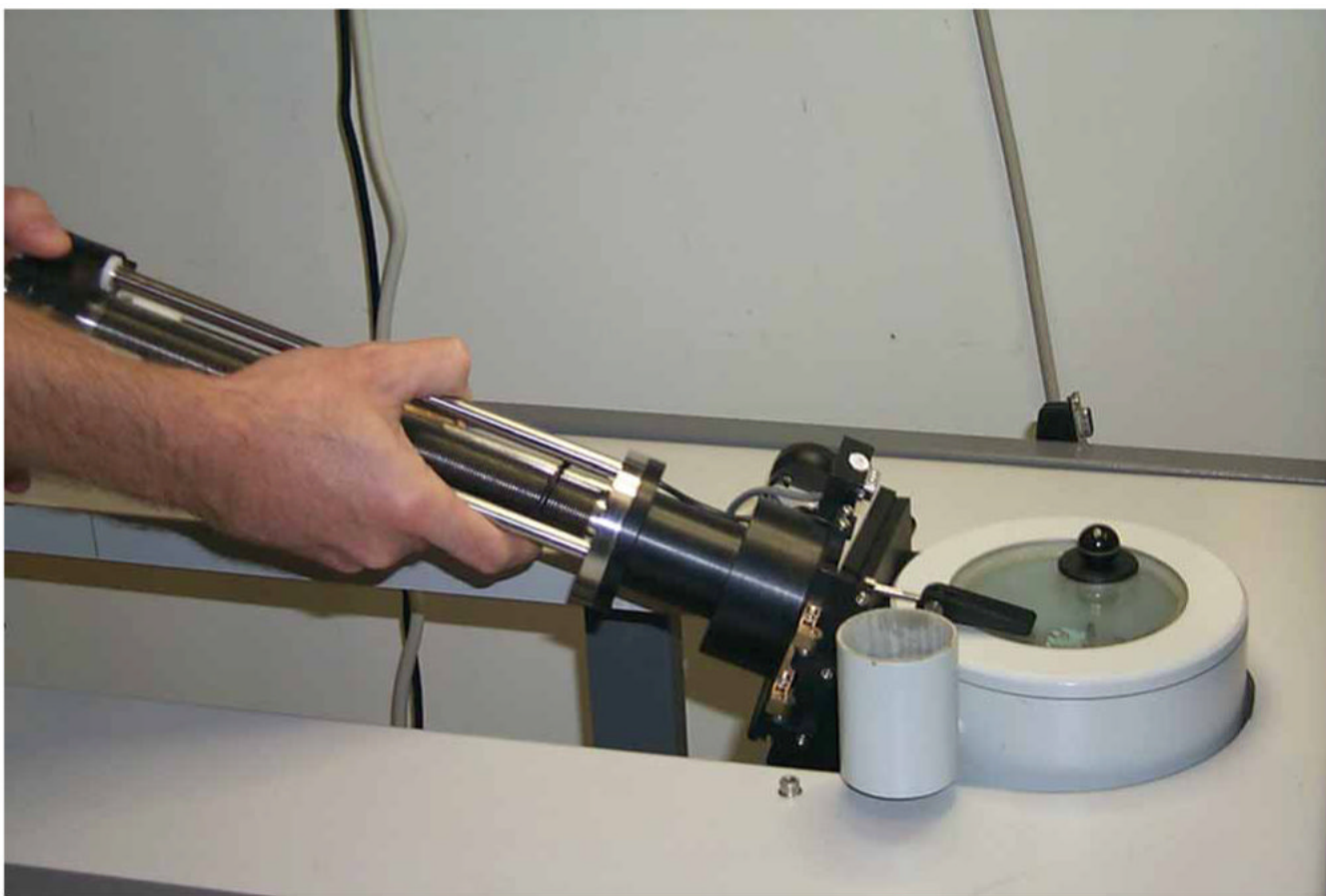
Figure 6. MSC being mounted on transfer station.
