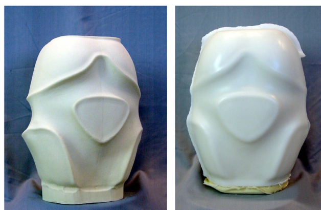
Figure 2 Foam model of the physio-logic™ brace. After the anthropometrical data (circumferential and longitudinal trunk measurements) are recorded, the foam model is milled from a blank hard foam block. This hard foam model is wrapped in a heated PE-plate, which is vacuumed to the models surface. The brace parts are cut from the PE-model and adjusted to the patient. The physio-logic™ brace is manufactured by Orthomed OT Services, Bad Sobernheim, Germany.
