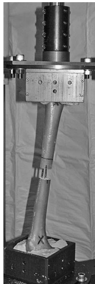
Fig. 1 Mechanical test setup for torsion and compression testing
