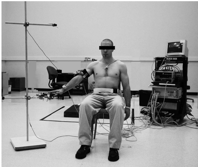
Figure 1. Patient testing setup. Each patient performed the humeral elevation and lowering tasks between the anthropometrically assigned hand triggers. We attached electromagnetic tracking sensors to the sternum, upper arm, forearm, and scapula (not shown in photograph) of each patient while he or she sat in a wooden chair. Adapted from the Journal of Shoulder and Elbow Surgery , 17(1), Scibek JS, Mell AG, Downie BK, Carpenter JE, Hughes RE, Shoulder kinematics in patients with full-thickness rotator cuff tears following a subacromial injection , 172–181, 2008, with permission from Elsevier. 10
