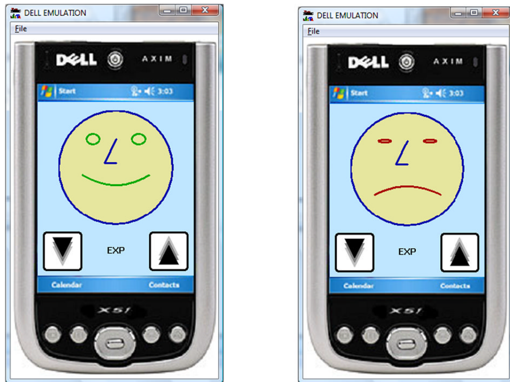
Figure 1. Sample facial impressions produced by the Computer Face Scale as implemented on a hand-held computer. Animated changes are produced by depressing the ‘up’ (smile) and ‘down’ (frown) arrows on the screen using a stylus, fingers or thumbs Figure A.1. Illustration of the computational method used to generate degrees of smiling and frowning by the Computer Face Scale.
