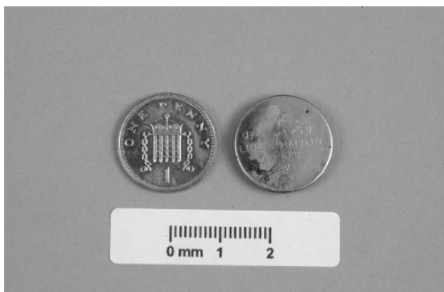
Figure 3 Comparative image of a one penny coin and a CR2032 button cell.
