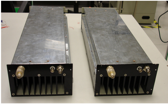
FIG. 4. a: Two ultra-low output impedance amplifier prototypes. b: Each amplifier is consisted of three amplification stages
