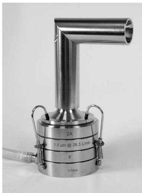
Fig. 1. Copley fast screening Andersen impactor (C-FSA)
