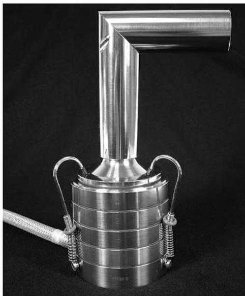
Fig. 2. “Trudell” fast screening Andersen impactor (T-FSA)
