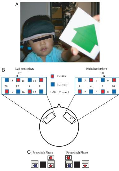
Fig. 1. Experimental settings. (A) A child with an NIRS probe. (B) The NIRS probe was attached to the inferior prefrontal area. Each channel consisted of 1 emitter optode and 1 detector optode. The ROI was located near F7/8, which corresponds to ch 15, 17, and 18 and to ch 6, 7, and 9, respectively. (C) An example of preswitch and postswitch phases.
