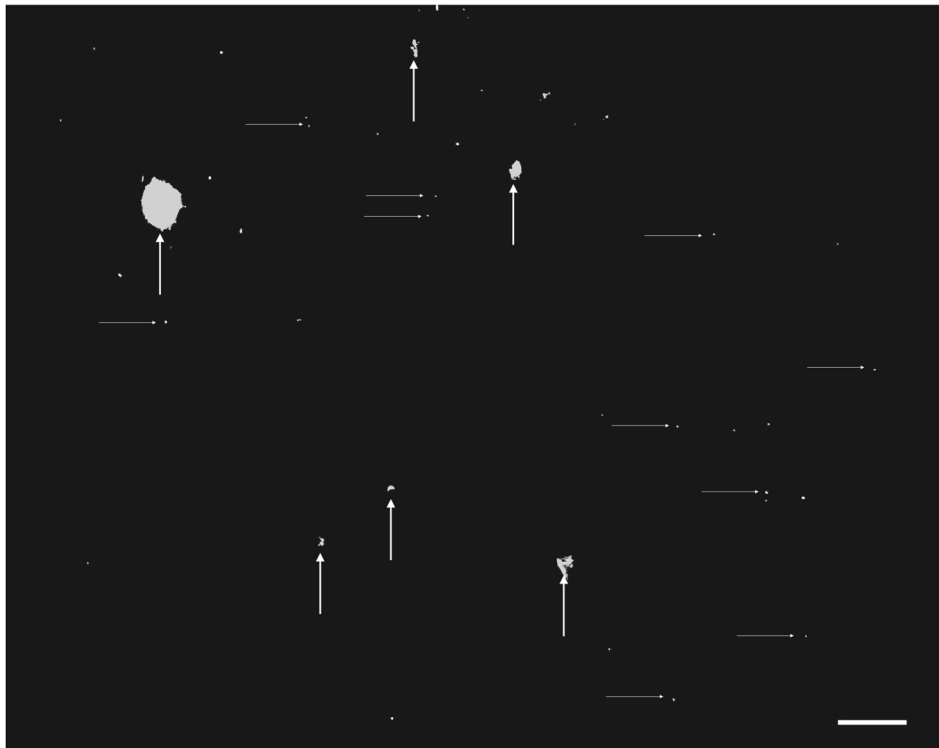
Fig. 3. Threshold processing of a typical fluorescent image. Large artifacts (vertical arrows) are recognized and removed from consideration, leaving the area fraction of fine particles (horizontal arrows) as the measure of delivery. Bar = 100 \mu\text{m} .
