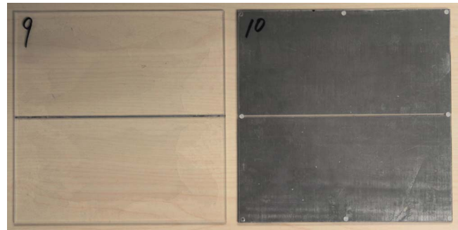
FIG. 2. The tools used for scatter line profile measurements. The left is for beam stop method and the right for aperture method.
