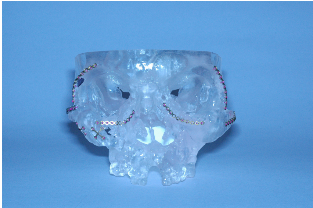
Figure 7. The titanium plates are adapted to the model aligning the screw-holes to the screw-hole markers (Frontal view)
