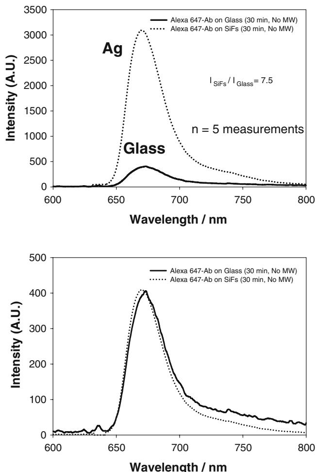
**Figure 4.** Emission spectrum of Alexa 647 on both SiFs and glass after 30-min incubation (top) and normalized to the fluorescence emission on glass (bottom). The spectra are the mean of five measurements on the respective surfaces.
