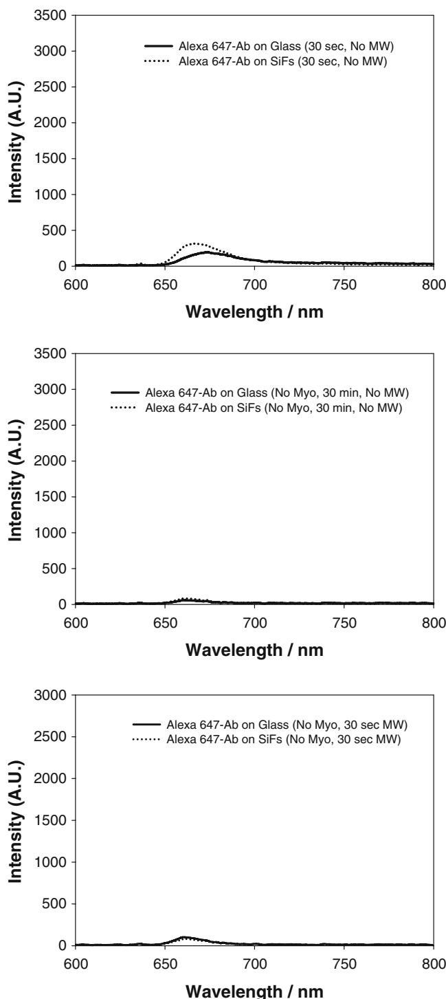
**Figure 6.** Control experiments: emission spectrum of Alexa 647 on both SiFs and glass after 30-s incubation at room temperature (with myoglobin; top), after 30-min incubation at room temperature (no myoglobin; middle), and after 30-s low-power microwave heating (no myoglobin; bottom).
