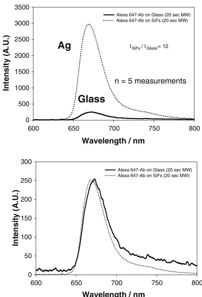
**Figure 5.** Emission spectrum of Alexa 647 on both SiFs and glass after 20-s low-power microwave heating (top) and normalized to the fluorescence emission on glass (bottom). The spectra are the mean of five measurements on the respective surfaces.
