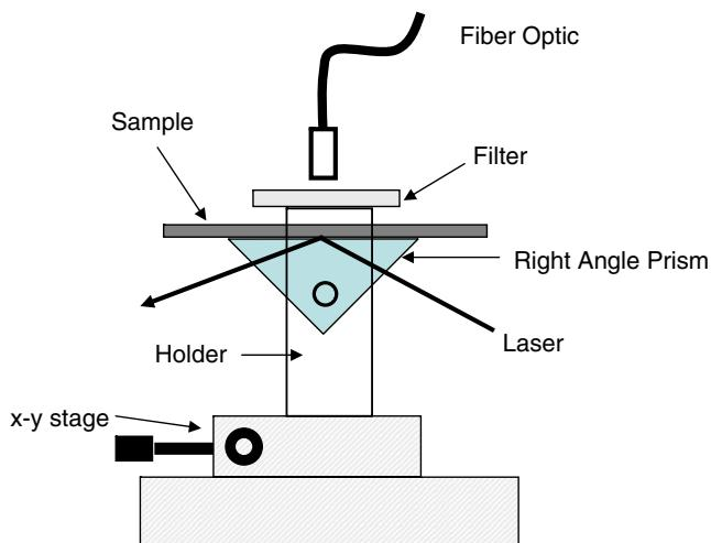
**Figure 2.** Total-internal reflection fluorescence geometry for myoglobin assessment.
