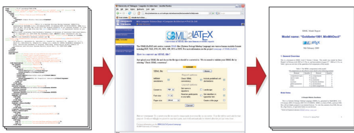
Fig. 1. Example workflow using the SBML2LATEX web service and SBML file BIOMD000000003.xml (available at http://www.ebi.ac.uk/biomodels ). After upload of an SBML file, several options allow customizing the output: MIRIAM annotations, an SBML consistency check or predefined unit declarations can be excluded, the desired file format can be selected; the paper size can be set to the US formats letter, legal or executive as well as to the European formats DIN A0-9 and the page orientation can be switched to landscape (especially important if the report contains fractions with very long denominators, where no automatic line break can be inserted). Several other options influence the layout of the report, e.g. names can be used in equations instead of identifiers, which can be displayed in typewriter or roman font. When the user clicks on the ‘convert’ button, the report file is generated and accessible for download.
