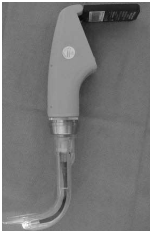
Figure 2 Photograph of the AWS® laryngoscope. The device is held in the left hand and passed into the mouth over the tongue, and the tip is placed under the epiglottis.
