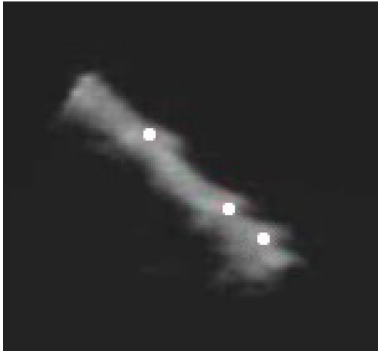
Figure 5. 3D Ultrasound image of an instrument with white dots indicating tracked passive markers.
