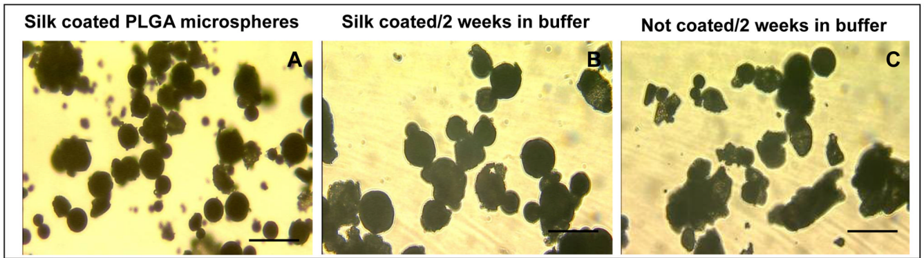
Fig. 2. Stabilization of PLGA microspheres by silk coatings. Silk coated PLGA microspheres had a spherical shape when suspended in PBS buffer, pH 7.2 (A). Most microspheres remained spherical shape after two weeks incubation at 37°C (B). Most control microspheres without coating lost their spherical morphology due to degradation after two weeks incubation at 37°C (C). Bar indicates 200 µm.
