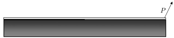
Figure 1. An elastic thin film adhering on a surface subjected to a peeling force. The film resembles a spatula pad with plane-strain Young’s modulus E=2 GPa, Poisson’s ratio \nu=0.3 and thickness 5 nm. The system is under plane strain with a unit width in the out-of-plane direction. The adhesion energy across the contact interface is taken to be 0.01 \text{ J m}^{-2} and the theoretical strength of adhesion is 20 MPa.
