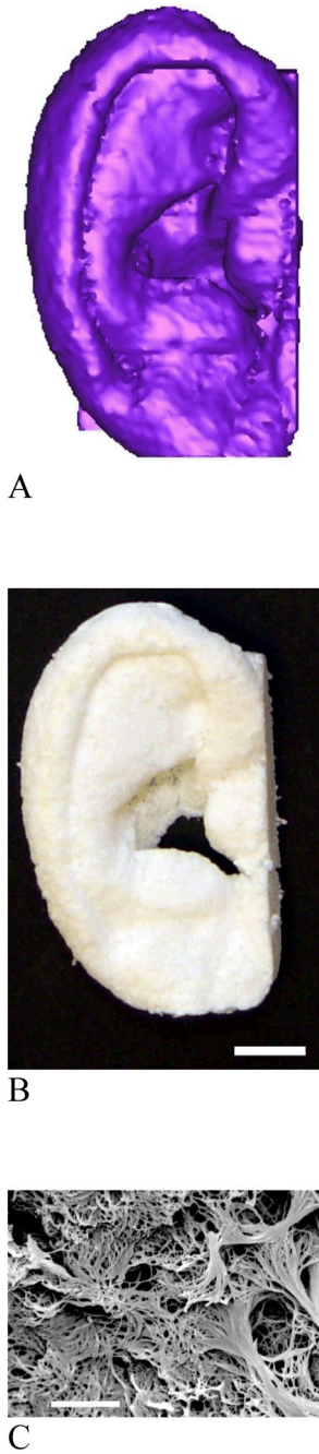
Fig. 4. Nanofibrous scaffolds created from 3D medical images and a phase-separation technique. (A) human ear template reconstructed from histological sections; (B) resulting nanofibrous scaffold of the human ear (scale bar: 10 mm); (C) the nanofibrous pore wall morphology (scale bar: 5 \mu\text{m} ). From Chen et al.[39] Copyright © 2006 by Elsevier. Reprinted with permission of Elsevier.
