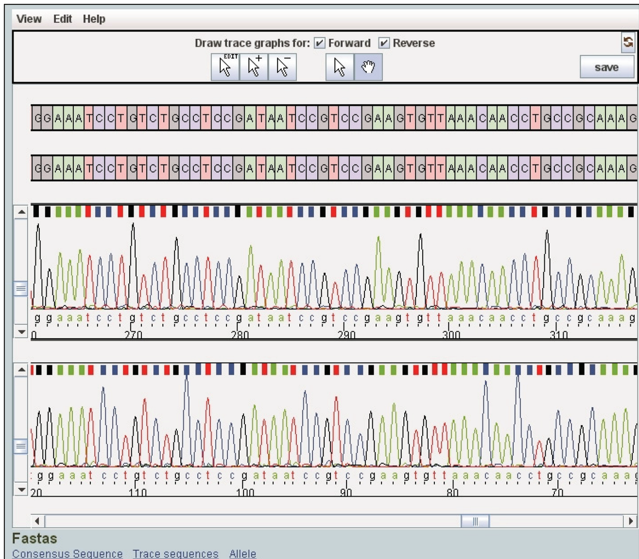
Figure 3. The trace viewer and editor applet. The consensus sequence acts as a backbone when aligning the allelic sequence and the traces. The applet tools allow users to (1) alter the amplitude of the traces, (2) edit the consensus sequence, (3) insert/delete consensus sequence nucleotides, (4) undo/redo any action and (5) save a modified consensus sequence. Sequences of interest are embedded below the applet so that they can be copied and pasted.
