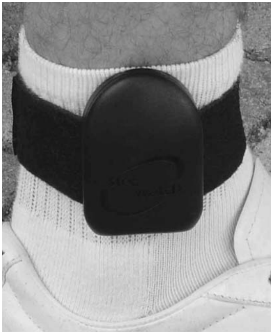
Fig. 1 A photograph shows the StepWatch™ Activity Monitor (SAM) worn at the ankle.
