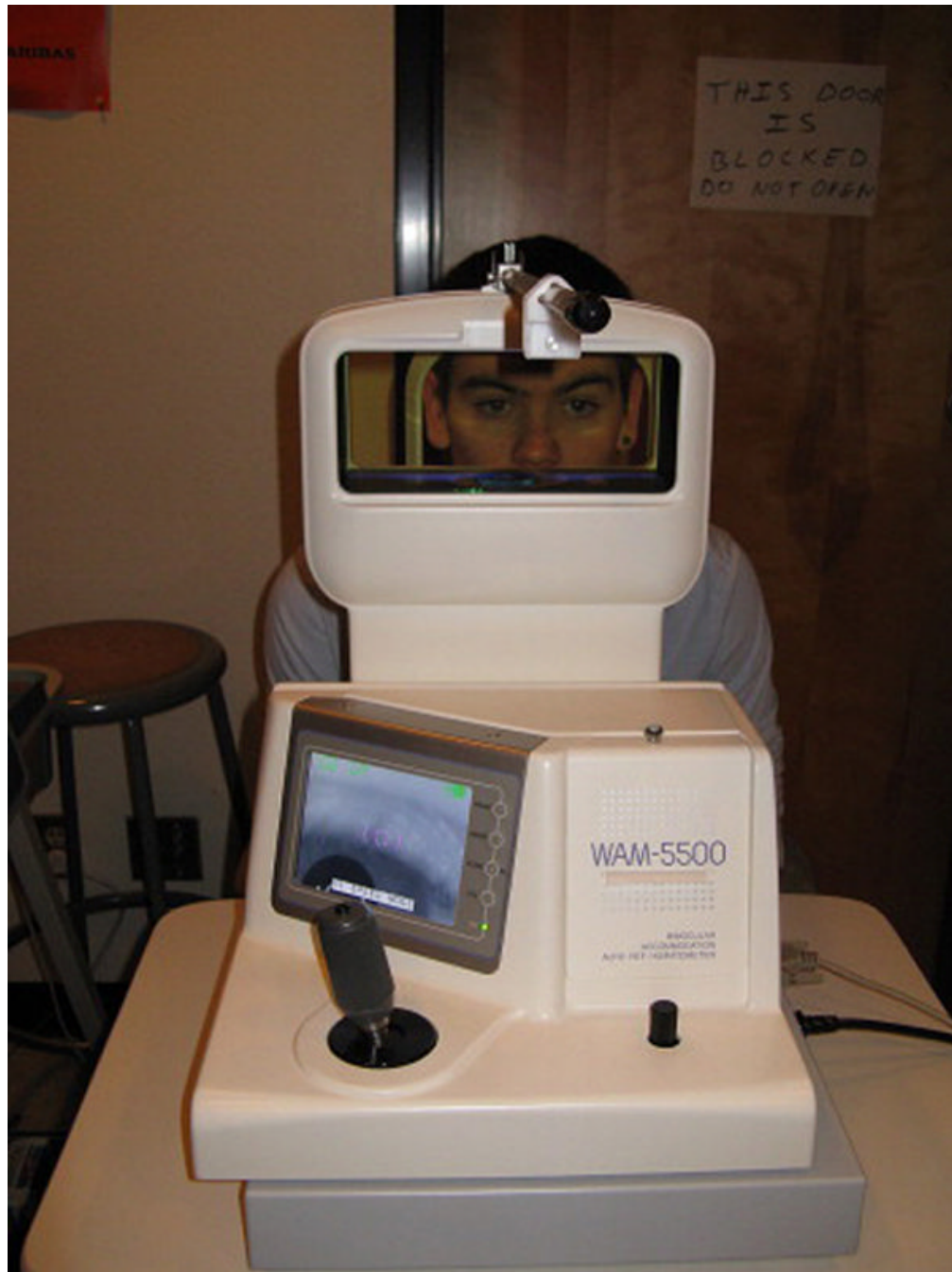
Figure 1. The WAM-5500 accommodation device. The subject (seated in back) looks through a screen at a target (not shown). The screen at the bottom left shows the subject's eye. The joystick is used to center the eye for obtaining measurements.
