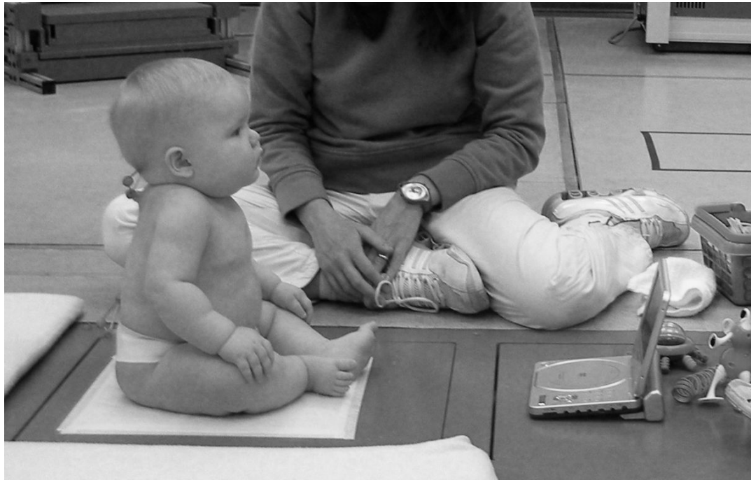
Figure 1. Position of infant during data collection. The infant is sitting on the top of a force plate while a DVD player is in front of the infant for maintaining a calm and relaxed state.
