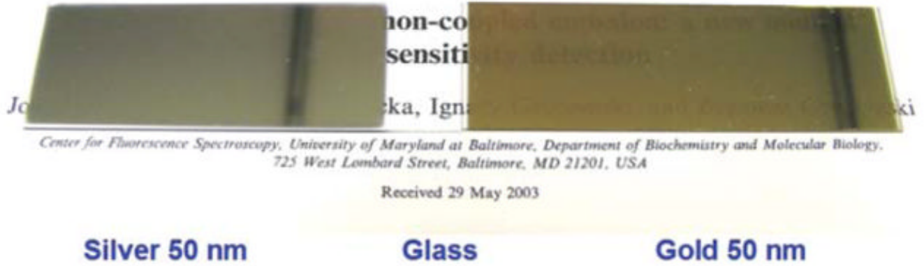
Fig. 32. Photograph of silver (left) and gold films (right) used for SPCE.
