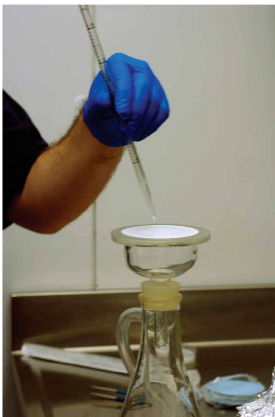
Figure 4. Creating filter culture from batch culture (Step 2A(vi)). Batch culture is slowly and evenly dripped onto a filter membrane, which sits on a sintered support base residing on top of a vacuum flask.
