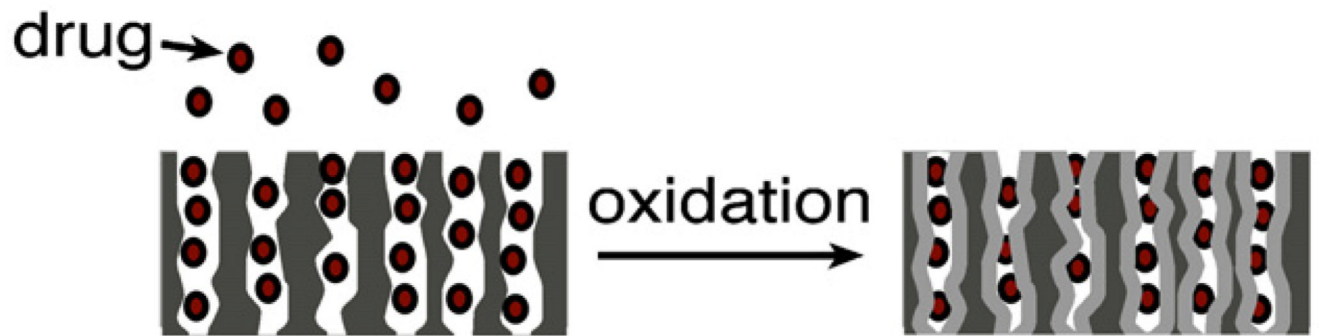
Fig. 4. Building a bottle around a ship. A molecular or nanoparticle payload can be trapped by partial oxidation of the porous Si host layer. Oxidation produces a volume expansion ( \text{Si} to \text{SiO}_2 ) that shrinks the pores, locking the payload in place. After [124]
