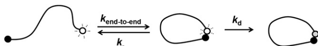
FIGURE 1 We have measured the end-to-end collision rates of single-stranded DNA using a long-lived luminophore (a ruthenium tris(bipyridine) derivative) and an electron-accepting quencher ( n -methyl- n' -ethyl viologen or DABSYL). The open and shaded circles represent the excited and ground states of the luminophore, respectively, and the solid circle represents the quencher. These constructs allow us to estimate collision rates from the reduction in the excited-state lifetime of the luminophore induced by the quencher. Specifically, when quenching occurs with high efficiency, k_d is significantly greater than k_- , and the quenching rate reports on the end-to-end collision rate ( k_{\text{end-to-end}} ) (see Eq. 1).
