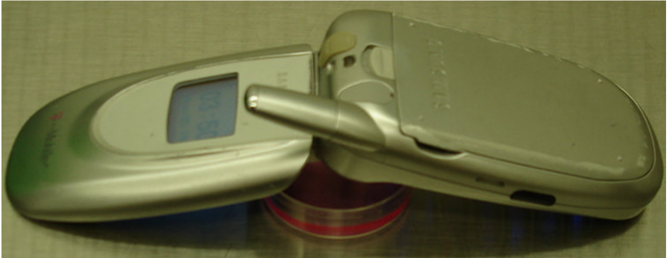
Fig. 1. Photograph of the method used to expose cultured cells to cell phone RF/MW radiation. The photograph shows a primary neuron culture in a 35 mm Petri-dish containing 2.0 ml medium. A cell phone in “stand-by” or “on” mode was placed on top of the petri-dish as shown.
