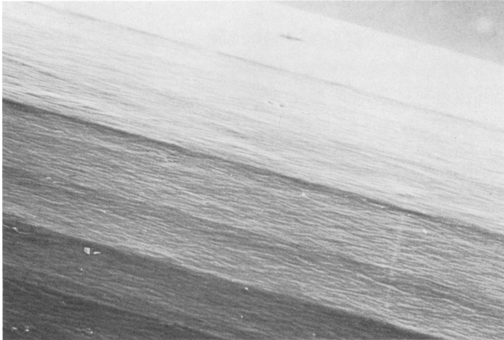
FIG. 1. SEM of unused sterile PVC catheter surface (magnification, \times 100 ).
