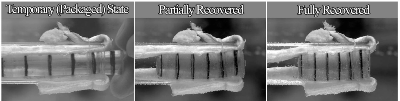
Figure 1. Demonstration of a shape-memory polymer cylindrical device expanding for soft tissue fixation. Note: Black lines were drawn for visualization.
