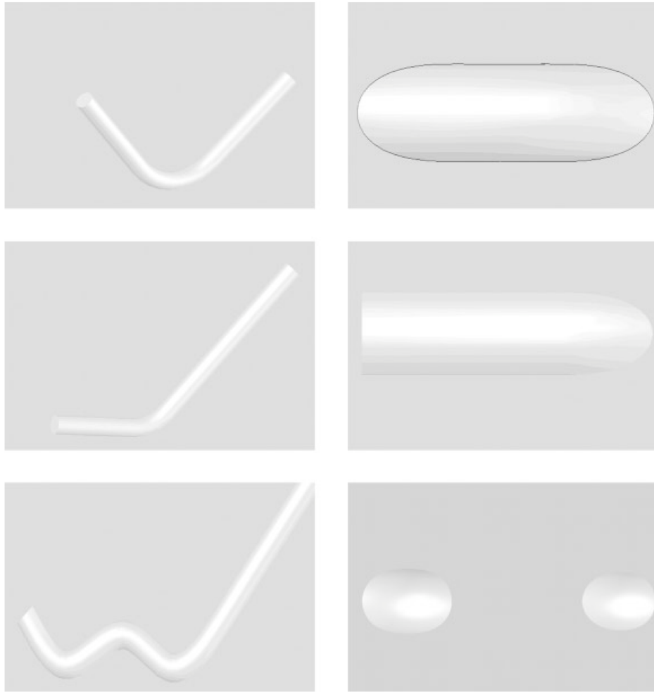
Figure 1. Different mandrel configurations used and corresponding shapes of the patches on the stent.
