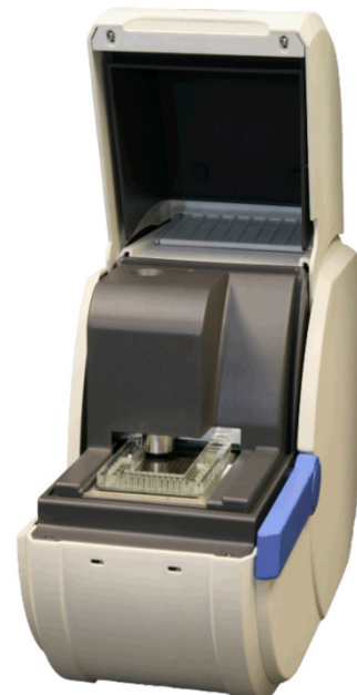
Figure 1. (Left) A fully assembled digital microfluidic multiwell plate cartridge (8.55 cm × 12.78 cm); (Right) the control instrument (20.32 cm W × 33.02 cm H × 53.34 cm L)
