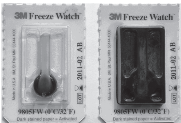
Figure 3. Freeze Watch™ indicators a used in a study of outside-the-cold-chain vaccine delivery in remote regions of western China
