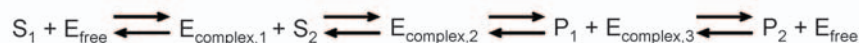
Figure 1. The elementary reaction mechanisms. Mechanisms used for the variety of different metabolic reactions. Reactions modeled as 1 substrate to 1 product: HPr, EIIA, Pgi, Tpi, Gpm, Eno, Pgl, Rpe, Rpi, Pta, Ppc, Fum, Sdh, recycle reactions of ATP, NADH and NADPH. 2 substrate to 1 product reactions: EIIBc, AroG fb . 1 substrate to 2 products: EI, Fba, Pfl. 2 substrates to 2 products: Pfk, Gap, Pkg, Zwf, Gnd, Tkt, Tal, Pyk, Pps, Ack, Mdh. doi:10.1371/journal.pone.0006903.g001
