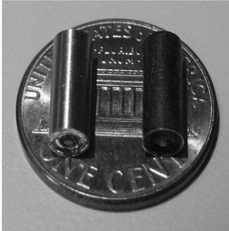
**Fig. 9.** Assembled miniature objective prototypes (oxidized and nonoxidized) on a US penny for size comparison.
