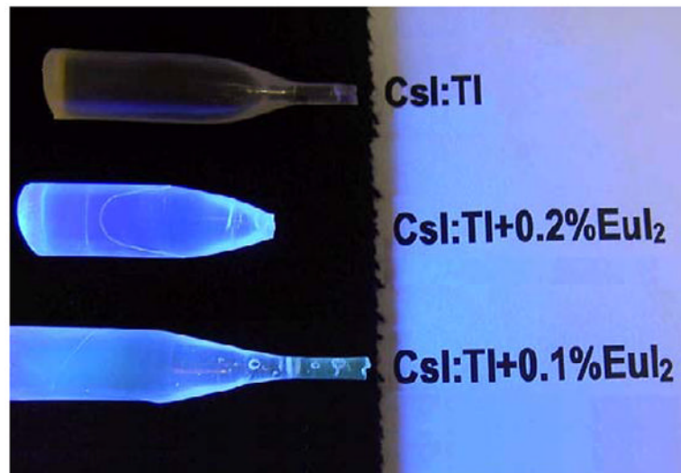
Fig. 1. A photograph of typical CsI:Tl and CsI:Tl,Eu single crystal boules grown at RMD, illuminated by their own UV-excited fluorescence. Note enhanced blue color, from emission added by Eu 2+ .
