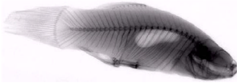
Fig. 6. Radiograph of a small fish taken using a 200- \mu\text{m} thick microcolumnar CsI:Tl, Eu film. Note well-resolved fine bone structure ( <100\ \mu\text{m} ) and excellent contrast between the background tissue and the air sacs.
